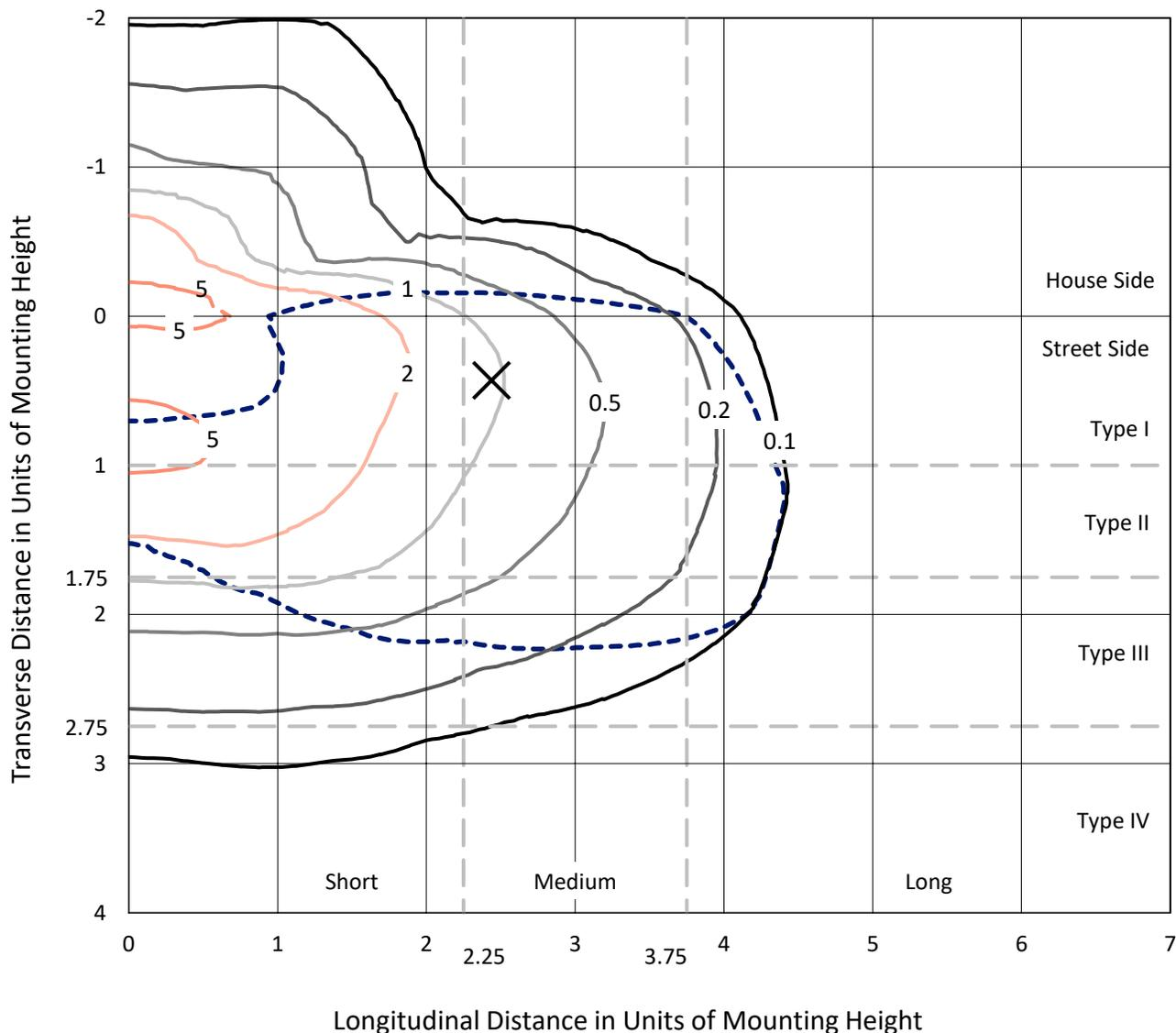
Based on 20 foot mounting height. Maximum calculated value = 6.3 fc
