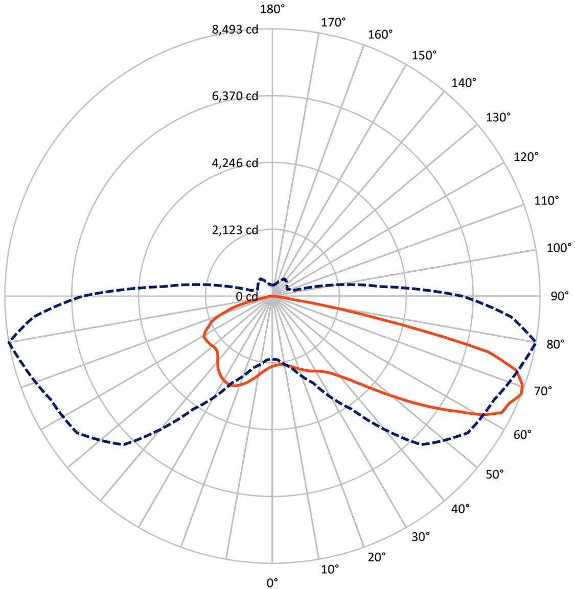
— Vertical Plane Through 80-Deg Lateral      - - - Horizontal Cone Through 68-Deg Vertical
